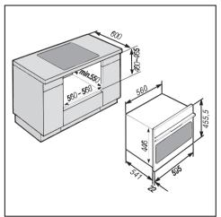
If fitted underneath a hob, the installation instructions for the hob must also be taken into account.
